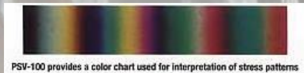
PSV-100 provides a color chart used for interpretation of stress patterns
